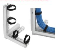
The ProLine Frame VELCRO® Tie-Down Bracket provides an easy means to secure and bundle cables using any of the frame's rectangular holes. The bracket can be positioned parallel or perpendicular to the frame and needs no tools to install—just push into any hole and twist to fasten. Proper bend radius is easily maintained with the flexible Velcro tie-down, plus it provides easy initial and future cable installations. Bracket is made of a durable plastic. Both tie-down and bracket are black.
