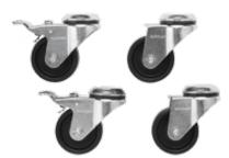
A set of four casters (two locking, two non-locking) that mount directly to the bottom of a ProLine frame, 0-mm or 100-mm Solid Base or a Console. (**Do not use on plinth bases.**) Casters elevate the enclosure 110 mm (4.33) when installed. Caster frames are plated steel with ball-bearing pivots. Caster wheels are made of a black polyamide material. Kit includes M12 mounting hardware.
